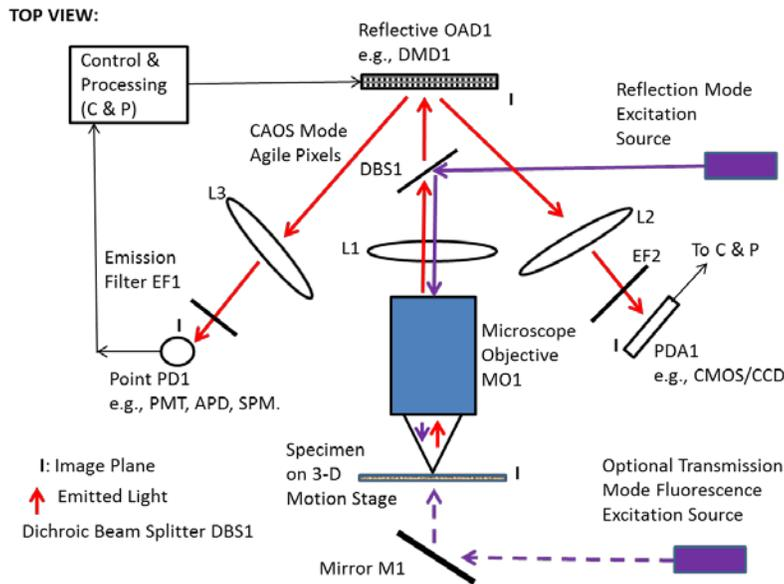
Fig.11. CAOS Smart Fluorescence Microscope/Nanoscope.
