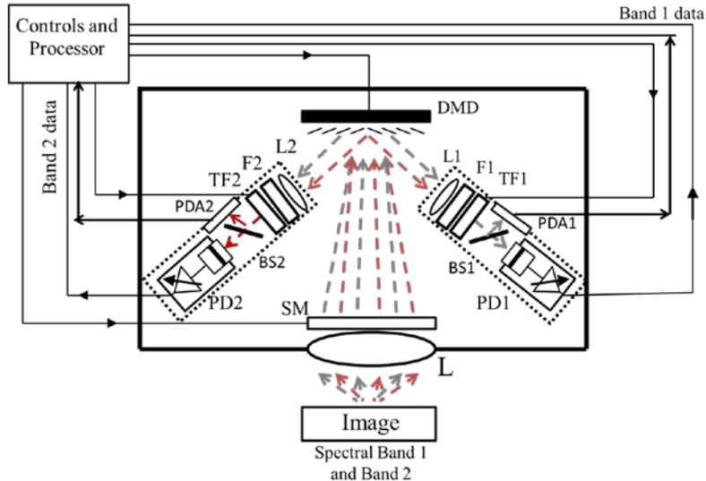
Fig.8. CAOS camera design for simultaneous dual-band imaging. F1/F2 are fixed broadband filters. TF1/TF2 are tunable optical filters. PDA1/PD2 are Photo-Detector Array Devices. BS1/BS2: Beam splitters. PD1/PD2: Point detectors. F1 allows band 1 passage and F2 allows band 2 passage [35].
