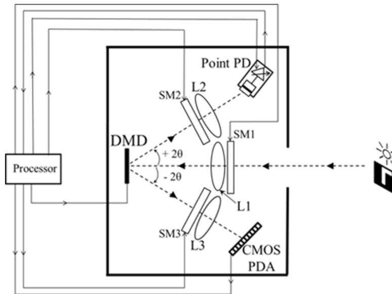
Figure 5: H-CAOS camera design using a DMD as the OAD and a CMOS PDA as the Hybrid (H) element. L1/L2/L3: Lenses. SM1/SM2/SM3: Smart Modules for light conditioning. PD: Photo-Detector with amplifier. [33]
