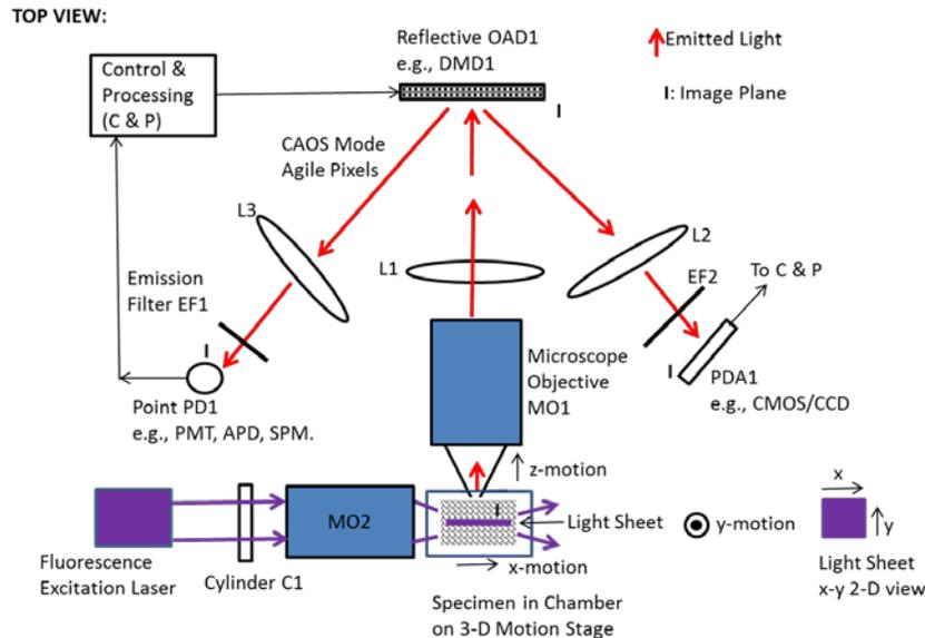
Fig.12. CAOS Smart Fluorescence Light Sheet Microscope/Nanoscope for 3-D Imaging.
