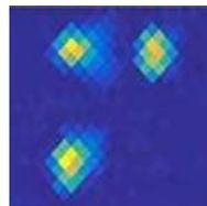
Fig.10. Visible band image captured by the Dual-band CAOS Camera using three visible LEDs and one SWIR LED target scene with LEDs arranged in a  $2 \times 2$  formation. The SWIR LED as expected is missing from the camera visible channel created image [35].
