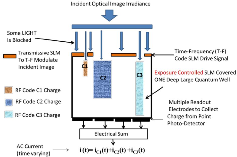
Fig.15. Basic operation of the point PD in the CAOS camera (shown is side view of sensor).
