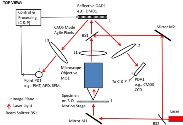
Fig.13. CAOS Smart Digital Holography Microscope.
