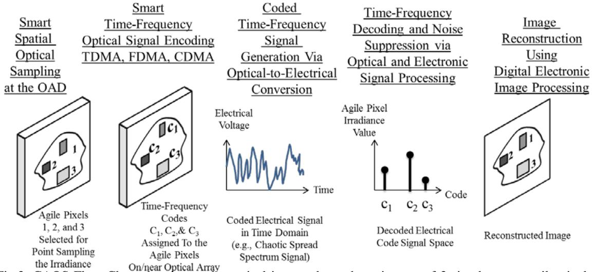
Fig.3. CAOS Flow Chart showing at the optical image plane, the existence of 3 simultaneous agile pixels of different sizes, locations, and shapes, each RF modulated with its own time-frequency code.
