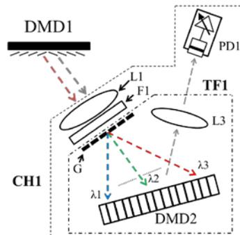
Fig.9 A possible DMD TF design for CAOS mode operations within the wavelength bands. G: Grating or wavelength dispersion element [35].
