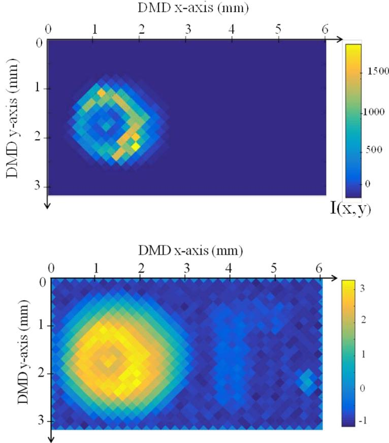
Figure 6. 82 dB HDR scaled irradiance map of the CAOS-mode acquired image in a linear (top photo: two faint targets not seen) scale and logarithmic (bottom photo: all three targets seen) scale. [33]
