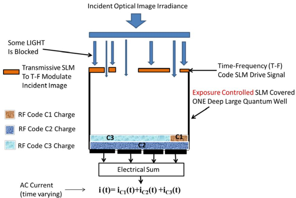
Fig.16 A more accurate illustration of Fig.14 showing how the 3 coded charge packets can fill the quantum bucket.
