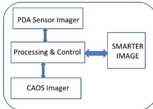
Figure 4: The CAOS Camera – A smart camera design combining CAOS and Photo-Detector Array (PDA) sensor (e.g., CMOS/CCD/FPA) technology.
