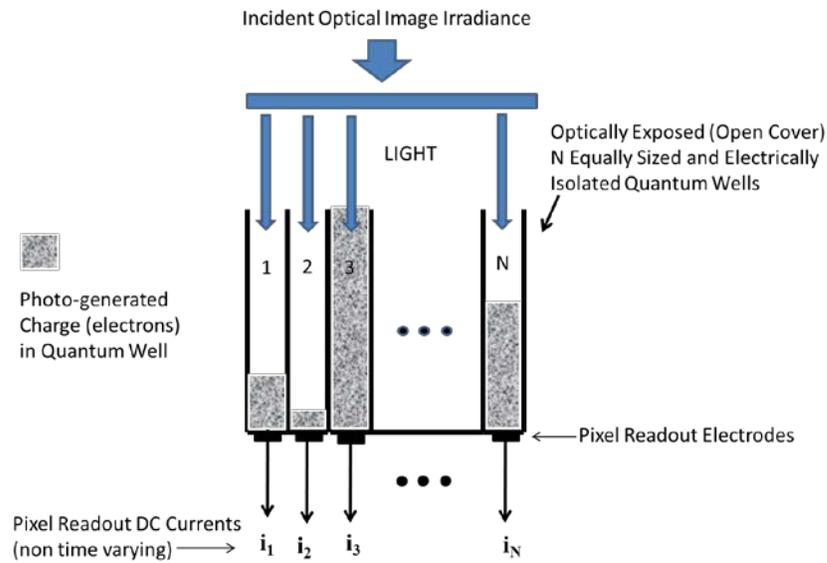
Fig.14. Operation of a classic PDA sensor (shown is side view of sensor).
